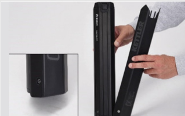
Figure 40: Pushing the battery cover onto battery
