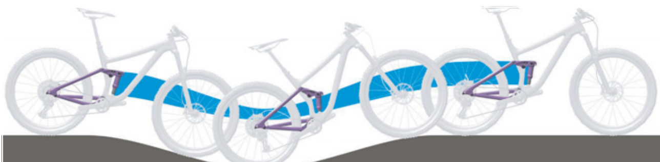
Figure 131: Excessively soft suspension in the rear frame damper on hilly terrain
