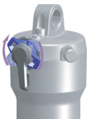
Figure 132: Changing compression adjuster to a harder setting
