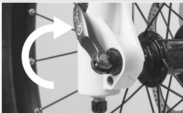
Figure 60: Closing the quick release
