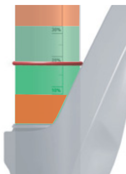
Figure 81: Mandatory sag range (green) and forbidden sag range
