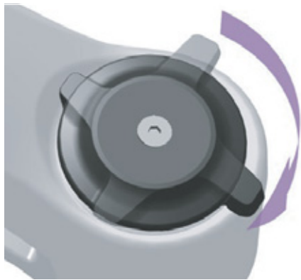
Figure 124: Changing compression adjuster to a harder setting
