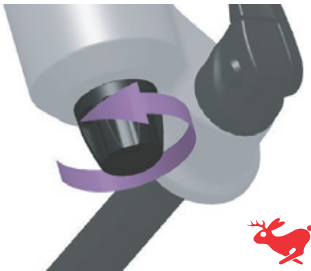
Figure 122: Turning rebound damper towards hare symbol
