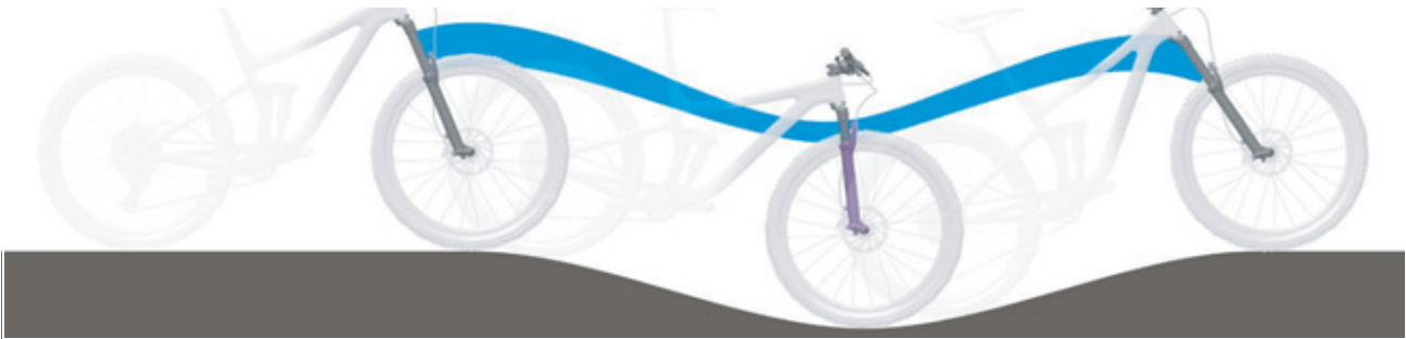
Figure 123: Excessively soft suspension in the suspension fork on hilly terrain
