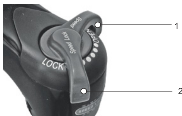
Figure 107: Suntour compression adjuster in open (1) and closed (2) position
