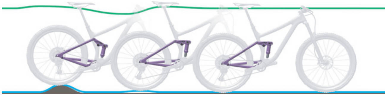
Figure 127: Rear frame damper rebounding too quickly
