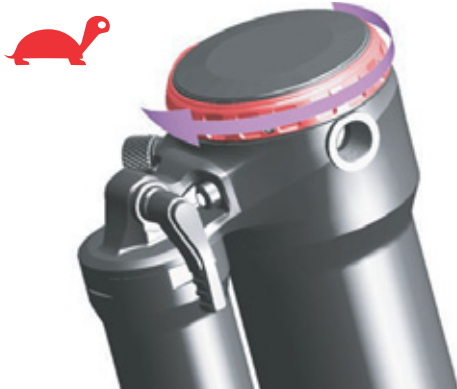
Figure 128: Turning rebound damper towards tortoise symbol
