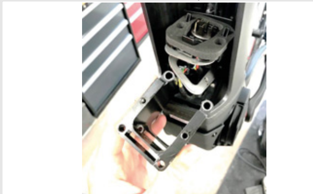
Figure 35: Pulling out the PowerTube adapter
