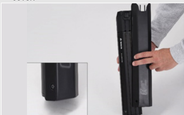
Figure 44: Pushing the battery cover onto battery
