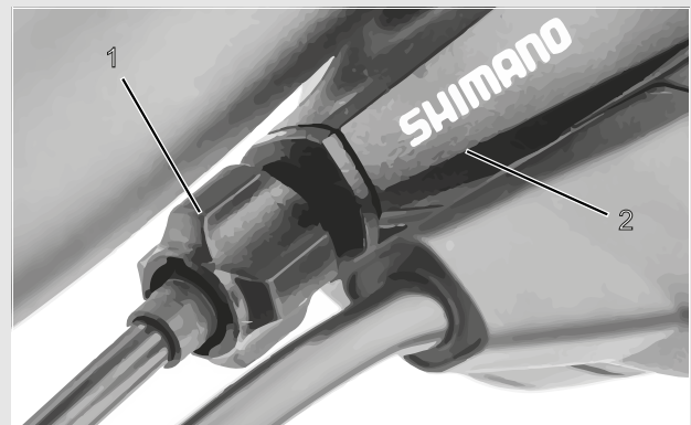
Figure 116: Adjusting sleeve (1) for the single-cable, cable-operated gear shift with shifter housing (2), example
