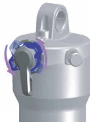
Figure 95: Changing compression adjuster to a softer setting
