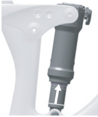
Figure 83: Moving the O-ring on the rear frame damper
