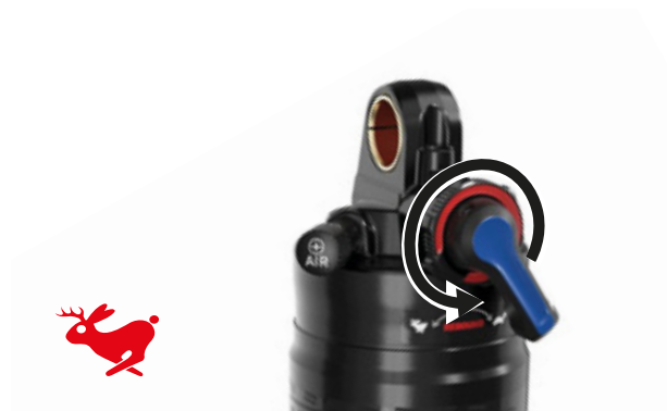
Figure 90: Increasing the rebound speed
