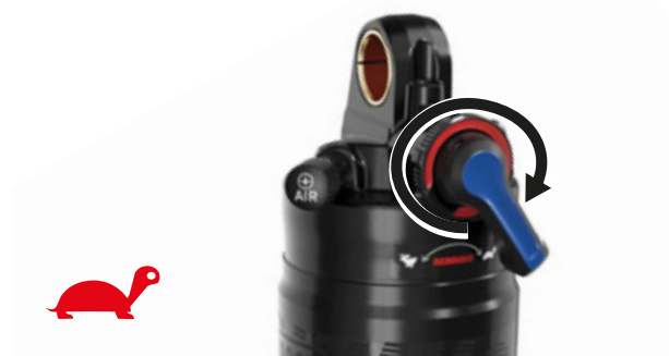
Figure 89: Reducing the rebound speed
