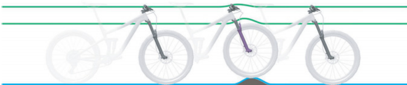
Figure 7: Optimum fork riding performance over bumps
