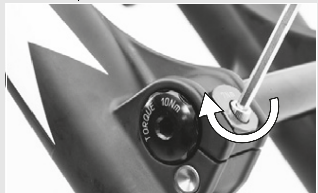
Figure 50: Tightening the securing clip
