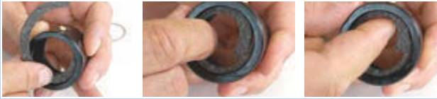
Figure 214: Inserting the felt ring
