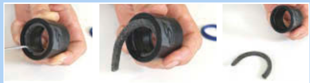
Figure 212: Removing the felt ring
