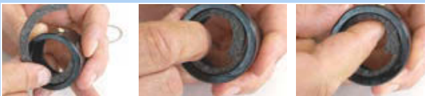
Figure 249: Inserting the felt ring
