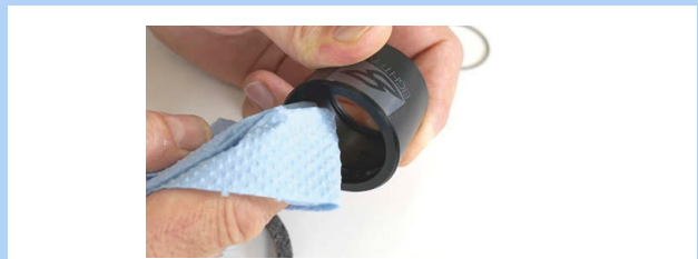
Figure 213: Cleaning the outer sleeve
