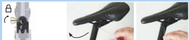
Figure 238: Closing the height adjustment
