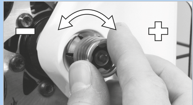
Figure 77: Adjusting the clamping
