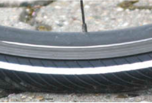
Figure 105: Correct tyre pressure. The tyre is barely deformed under the load of the body weight
