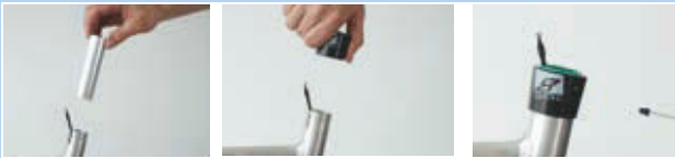
Figure 225: Fitting the slide bushing and outer sleeve
