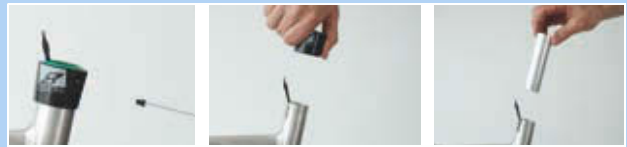
Figure 243: Removing the outer sleeve and slide bushing
