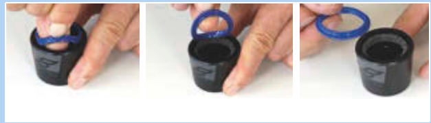
Figure 211: Removing the wiper
