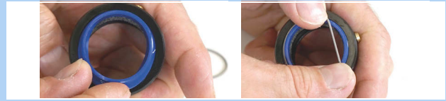
Figure 250: Inserting and fastening the wiper
