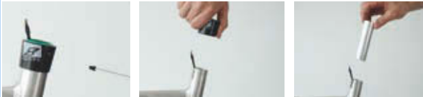
Figure 209: Removing the outer sleeve and slide bushing
