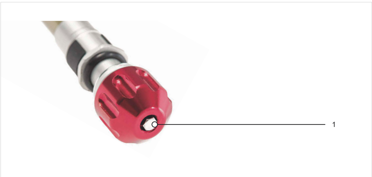
Figure 265: Example of SR SUNTOUR rebound adjuster (fork) (1)
