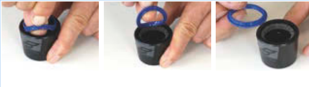
Figure 246: Removing the wiper
