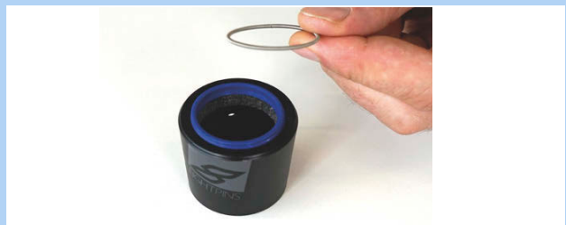
Figure 245: Removed spring washer
