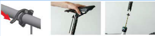
Figure 202: Pulling the seat post out
