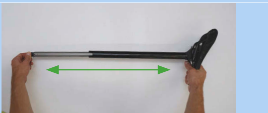
Figure 253: Pulling the seat post out
