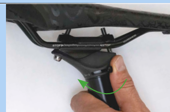
Figure 257: Closing the height adjustment
