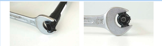
Figure 222: Securing against twisting
