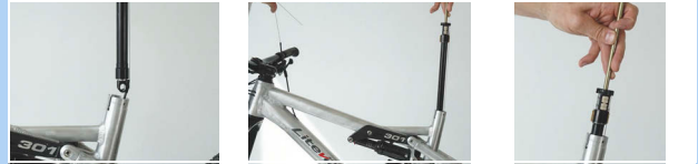
Figure 229: Fastening the cartridge valve cover
