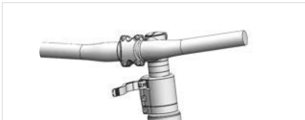
Figure 138: Example of All Up with open stem clamping lever
