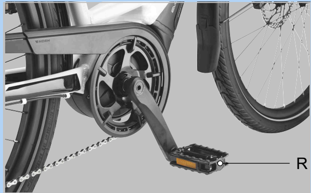
Figure 81: R-pedal in the right-hand crank arm
