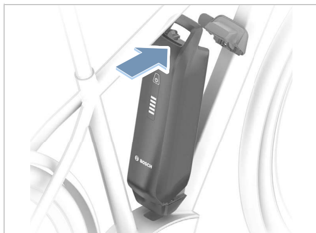
Figure 137: Closing the PowerPack battery upwards
