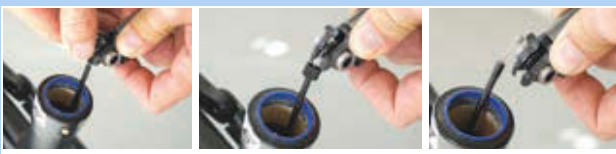
Figure 242: Removing the Bowden cable
