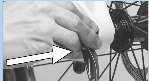
Figure 76: Inserting the quick release in the direction of the arrow
