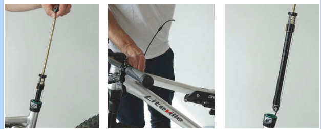
Figure 205: Pulling the cartridge out
