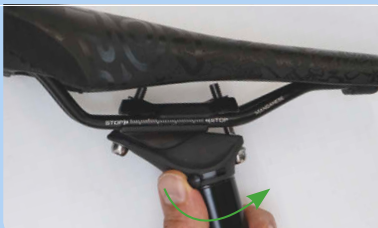
Figure 252: Opening the height adjustment
