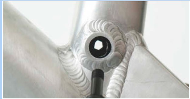
Figure 261: Hole in the Postpin interface
