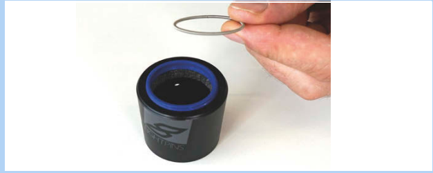
Figure 210: Removed spring washer
