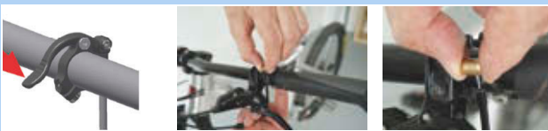
Figure 203: Removing the cartridge
