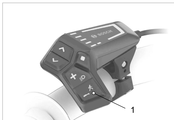
Figure 150: Position of push assist button (1)
