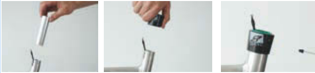
Figure 258: Fitting the slide bushing and outer sleeve
