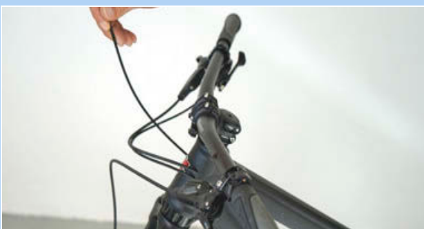
Figure 260: Attaching the end cap
