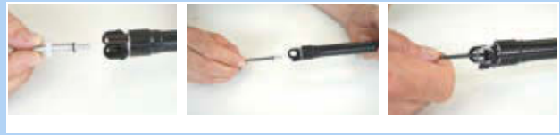
Figure 224: Fastening the cartridge valve cover
