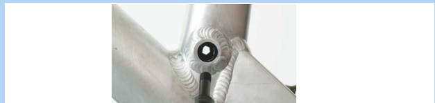
Figure 230: Fastening the cartridge valve cover
