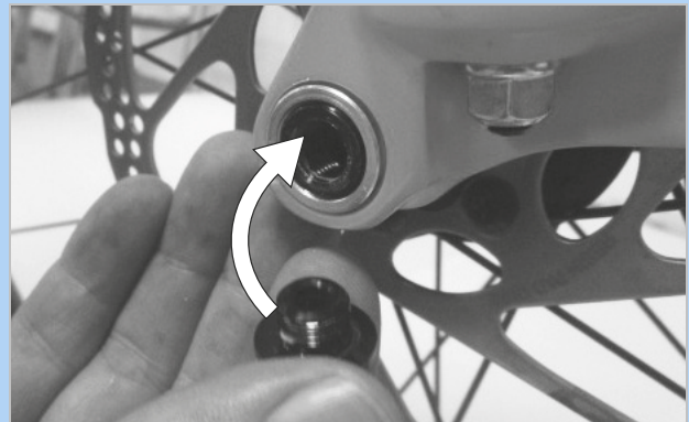
Figure 67: Inserting the securing screw
