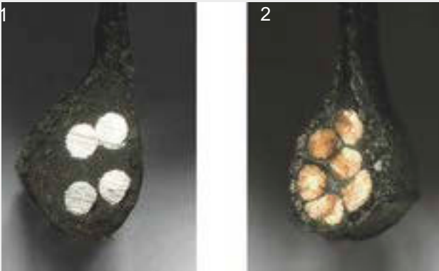
Figure 24: Steel bead core (1) and Kevlar bead core (2)
