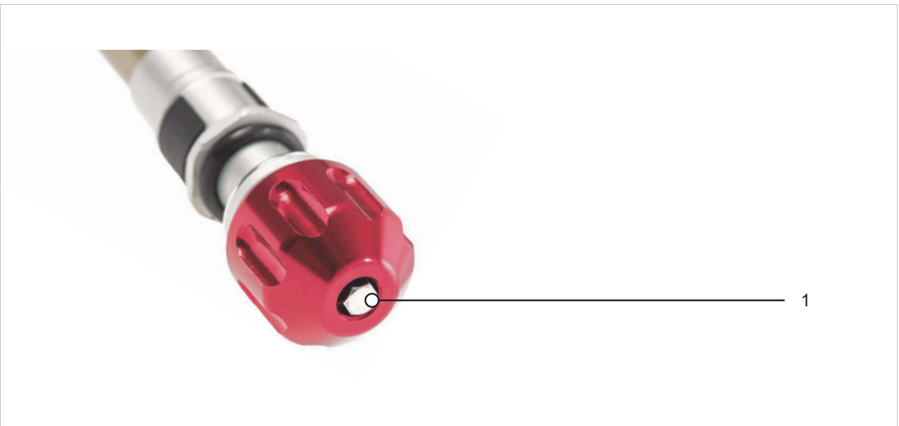
Figure 267: Example of SR SUNTOUR rebound adjuster (fork) (1)
