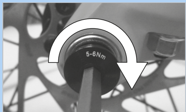
Figure 68: Tightening the securing screw
